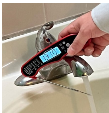
Photograph 13 (left): All-purpose thermometer registering a water temperature of 143.6 °F.
