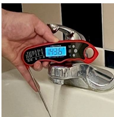
Photograph 13 (left): All-purpose thermometer registering a water temperature of 143.6 °F.
